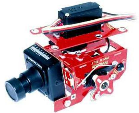
**Figure 1**, OSD camera setup for under carriage mounting.
