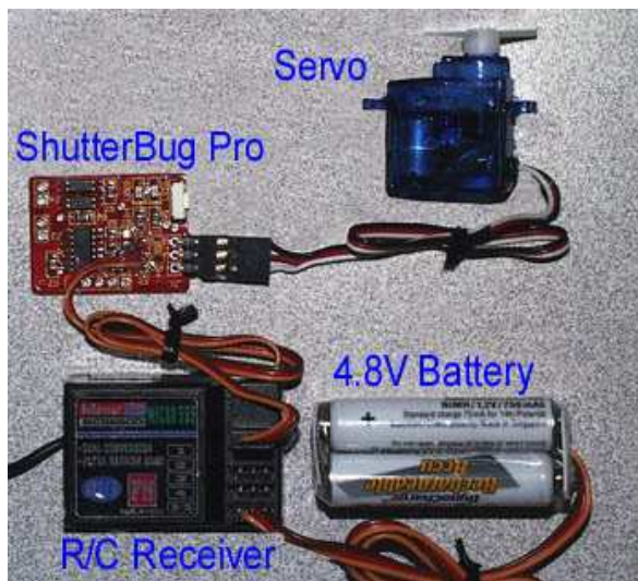
Figure 4, ShutterBug works with model R/C systems.
