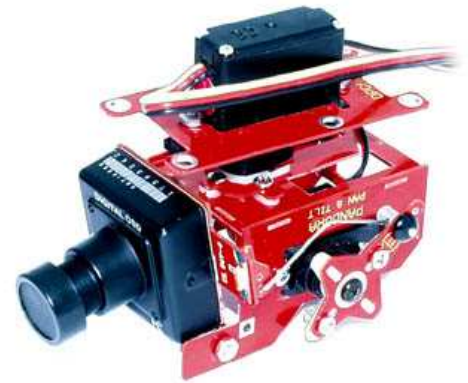
Figure 1 , OSD camera setup for under carriage mounting.
