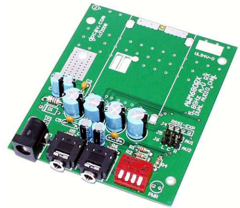
Figure 3 , Add the Switches and Jacks.
